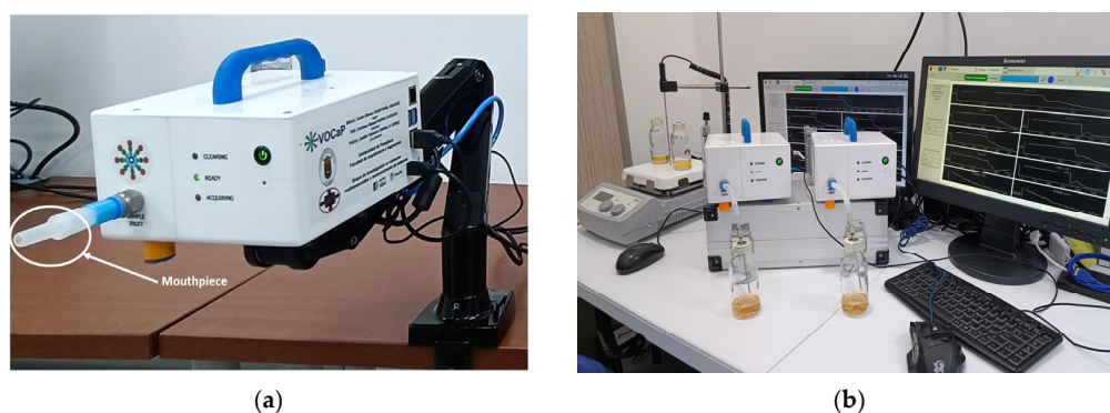
Figure 2. eNose System: (a) Sampling device for breath collection using a disposable mouthpiece, (b) Sampling protocol for urine collection generating a headspace.
