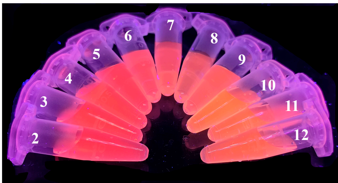
Figure S4. Photo of SiO 2 @Ag: ZIS QDs @ DMSNs aqueous solutions at different pH values under a 365nm fluorescent lamp.
