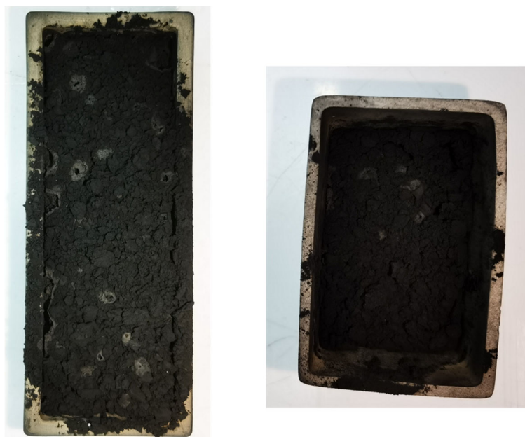
Figure S3: Graphene oxide black powder obtain after thermal treatments.
