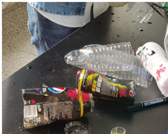
Figure S1: Plastic beverage bottles made of PET material are acquired, the hard parts at both ends are removed, and the thin middle section is cut into pieces.
