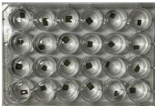
Figure S1. Image of the 24-well plate with the substrates on which the SOD assay was performed.
