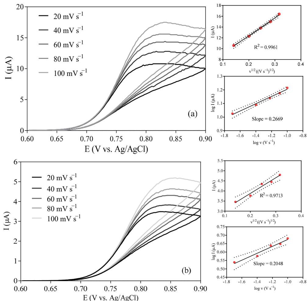
**Figure 5.** Cyclic voltammograms obtained at sensors (a) X1 and (b) X2 in 0.5 M H<sub>2</sub>SO<sub>4</sub> solution containing with 0.01 M paracetamol at different scan rates. Insert: log (I (μA)) vs. log (v (V s<sup>-1</sup>)) and I (μA) vs. v<sup>1/2</sup> ((V s<sup>-1</sup>)<sup>1/2</sup>). The dashed lines represent the 95% of confidence of data obtained.
