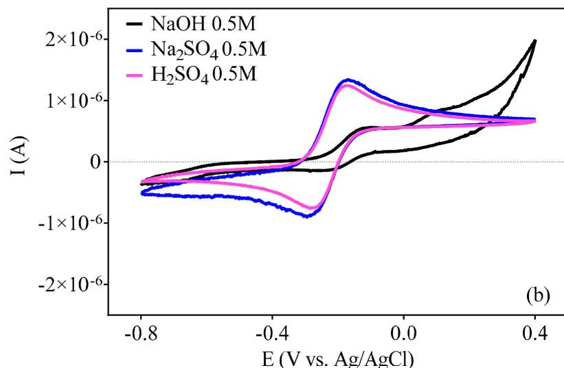
**Figure 1.** Cyclic voltammograms obtained in 0.5 M  $\text{H}_2\text{SO}_4$ , 0.5 M  $\text{NaOH}$ , and 0.5 M  $\text{Na}_2\text{SO}_4$  solutions adding 0.5 mM hexamine ruthenium trichloride ( $\text{Ru}(\text{NH}_3)_6\text{Cl}_3$ ) using the RC- and RGC-modified carbon paste sensors (a) X1 and (b) X2 electrodes, respectively. Scan rate =  $50 \text{ mV s}^{-1}$  and number of cycles = 10 cycles.
