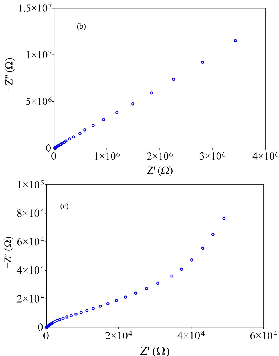
**Figure 4.** Nyquist plots for the investigated sensors: (a) X1 (RC-modified); (b) X2 (RGC-modified); and (c) X3 (pure carbon paste).
