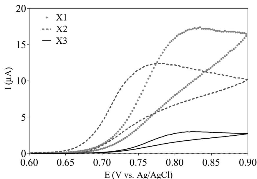
**Figure 2.** Cyclic voltammograms recorded on RC-(X1) and RGC-(X2) modified carbon paste sensors, and unmodified sensor (X3), in the presence of 0.01 M paracetamol (in 0.5 M  $\text{H}_2\text{SO}_4$ ); scan rate:  $50 \text{ mV s}^{-1}$ .
