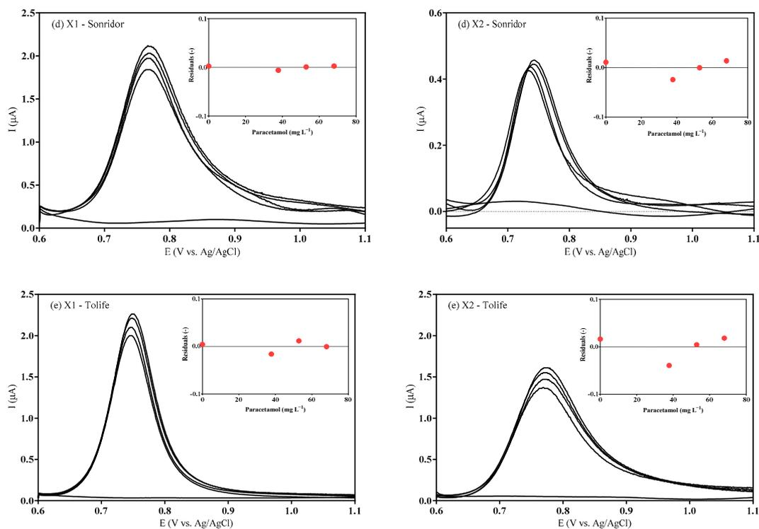
**Figure 7.** DPV curves for the five drugs analyzed with sensors X1 and X2: (a) Benegrip Multi Noite, (b) Doril Enxaqueca, (c) Naldecon Noite, (d) Sonridor and (e) Tofife. Insets: Graphics displaying weighted residuals for all detection measurements.
