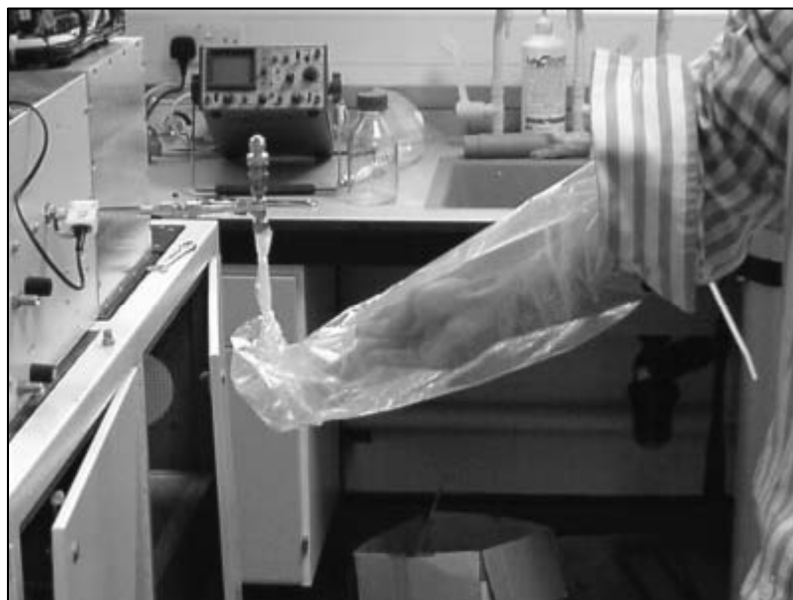
Figure 4. The sampling bag attached to the arm and the setup for SIFT-MS analysis of skin volatiles [128].
