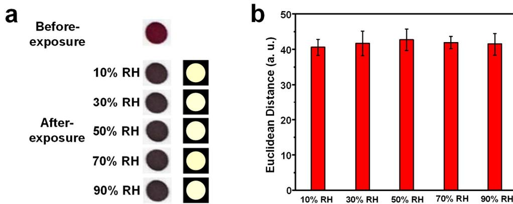
**Figure S3.** Humidity tests of microsphere-based sensors synthesized at 150 °C. (a) Before- and after-exposure images of the sensor spot and RGB difference profiles upon exposure of 1 ppm cyclohexanone with the 10%–90% relative humidity (RH), which is displayed in the color range of 3–10. (b) Sensor response to 1 ppm cyclohexanone at different levels of RH.
