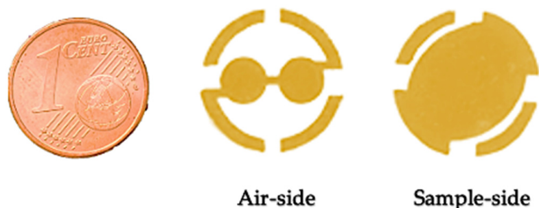
Figure 2. Self-made, dual-electrode design of QCMs (both air side and sample side).
