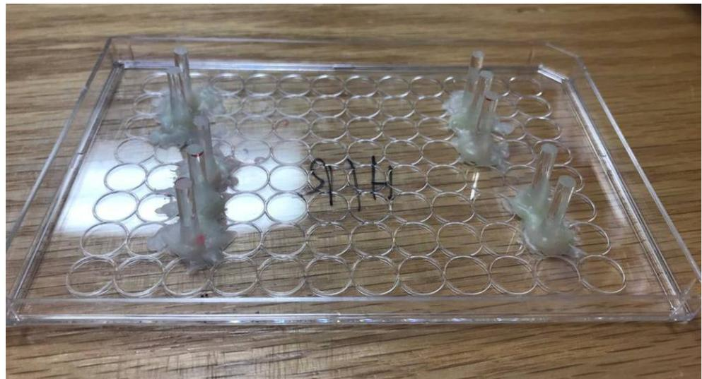
**Figure 3.** Image of the compression device. Plastic rods with 16 mm length and 3.175 mm diameter were fixed onto a lid of a 96-well plate.
