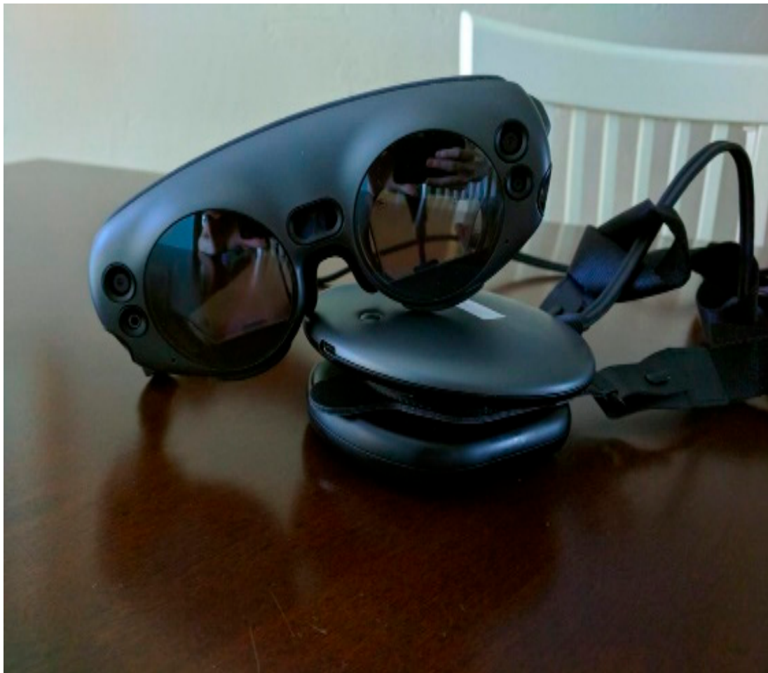
Figure 1. Magic Leap One™ kits include a headset, a portable computer/battery pack, and a controller. Source: University of Miami IT Department.
