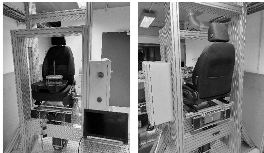
Figure 1. Original test equipment for biaxial loading.
