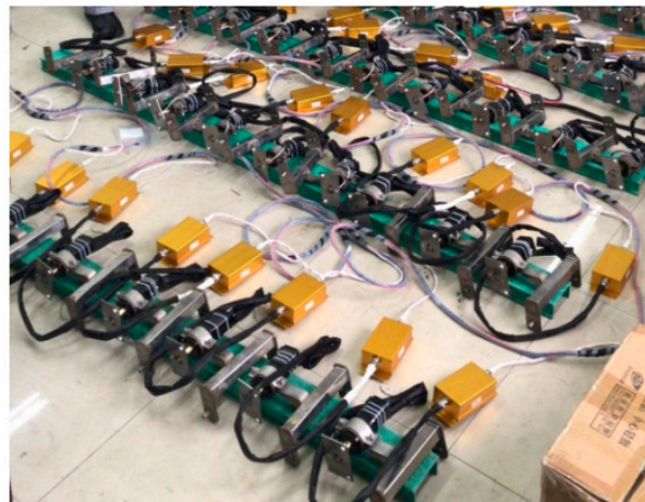
Figure 7. Schematic diagram of offline commissioning of anode rod measuring device.
