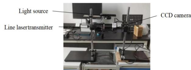
**Figure 12.** Experimental device.
