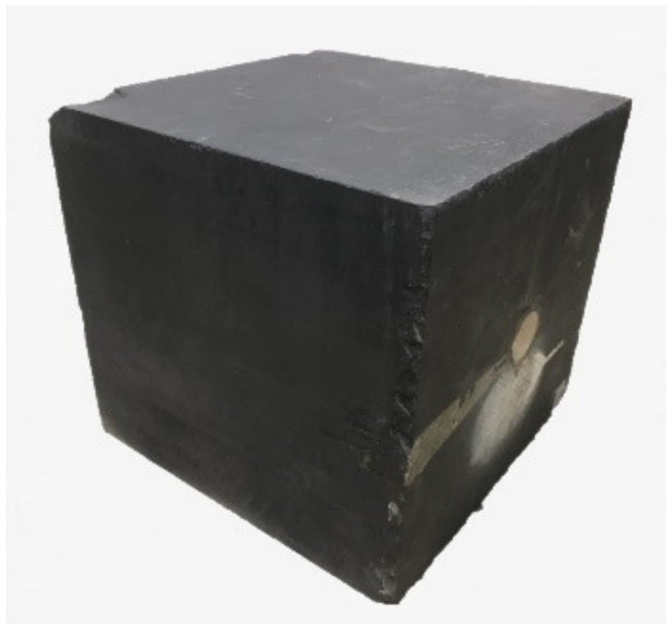
Figure 1. 30 cm × 30 cm × 30 cm cubic rock specimen.
