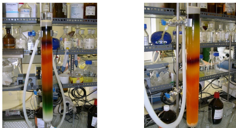
Figure 3. Column chromatography of an alga extract on modified silica gel.
