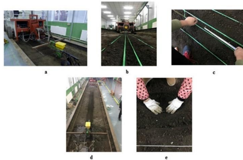
Figure 2. Soil bin test for covering. (a) seeding unit with covering discs; (b) artificial construction of soil furrow; (c) artificial sowing; (d) covering soils with precision seeding unit; (e) uncovering the seeds by hand.
