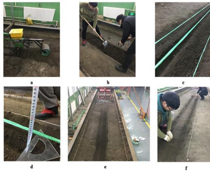
Figure 3. Soil bin test of compacting. (a) Soil sample preparation (soil loosening and testing firmness before each trial); (b) seeding unit with the compacting component; (c) artificial construction of soil furrow; (d) recording the positions of the seeds; (e) covering soil not disturbing the seeds; (f) uncovering the seeds after compacting.
