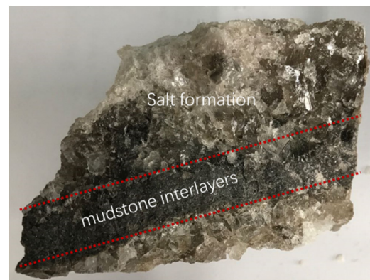
Figure 3. Multi-interlayer salt rock derived from well A.
