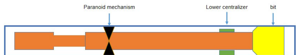
Figure 1. Schematic diagram of the new rotary steerable drilling system.
