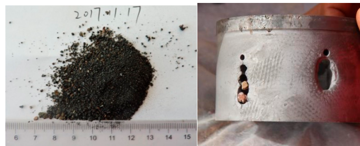
Figure 2. Sand sample and erosion diagram of nozzle cage.
