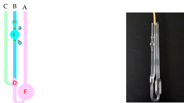
Figure 1. Ubbelohde viscometer. A—Air suspension pipe; B—Measuring capillary; C—Liquid injection pipe; D—Round pipe; E—Quantitative sphere; F—Liquid ball; G—Buffer ball; a—Upper score line; b—Lower score line.
