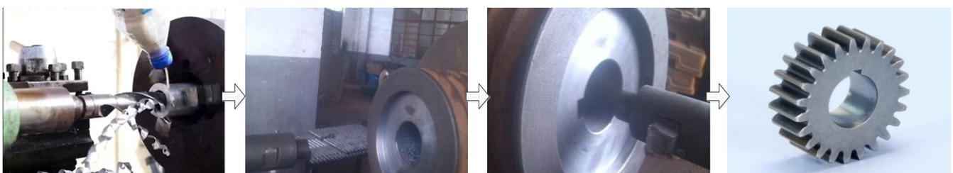
**Figure 2.** Stages of the gear during the manufacturing process.
