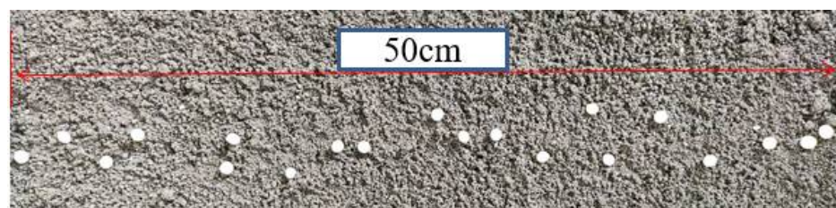
Figure 17. Distribution of soybean seed particles on the soil tray.
