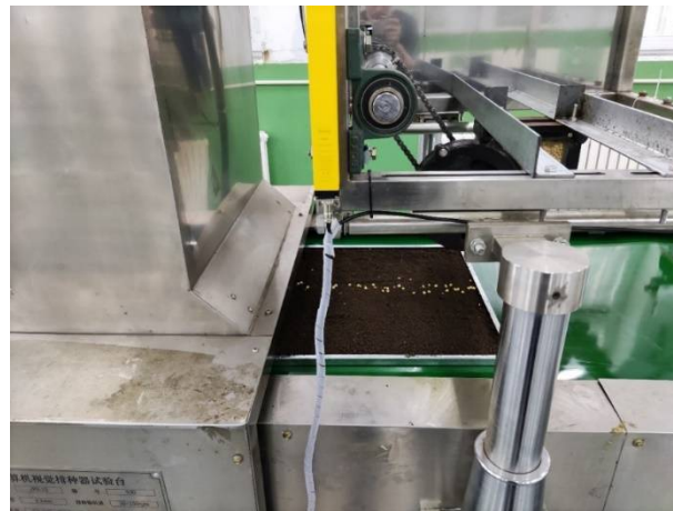
Figure 16. Computer vision seeding test bench.
