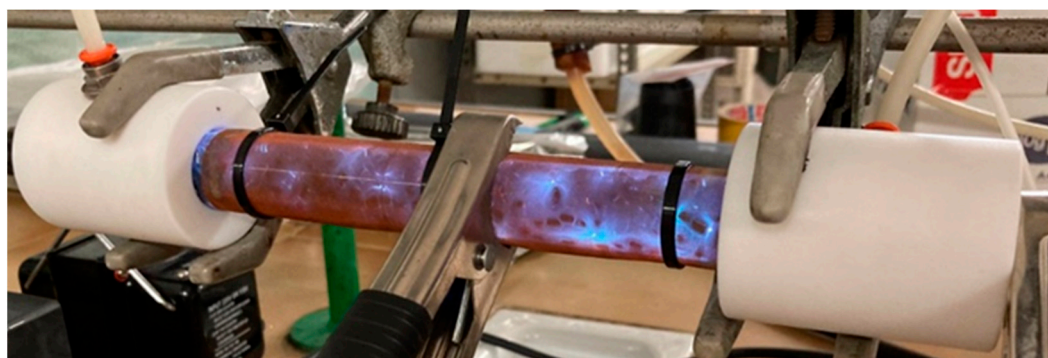
Figure 2. Picture of the NTP discharges across the DBD plasma reactor.
