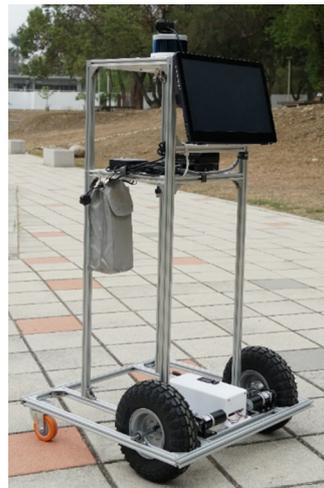
**Figure 22.** Remotely controlled mobile carrier.
