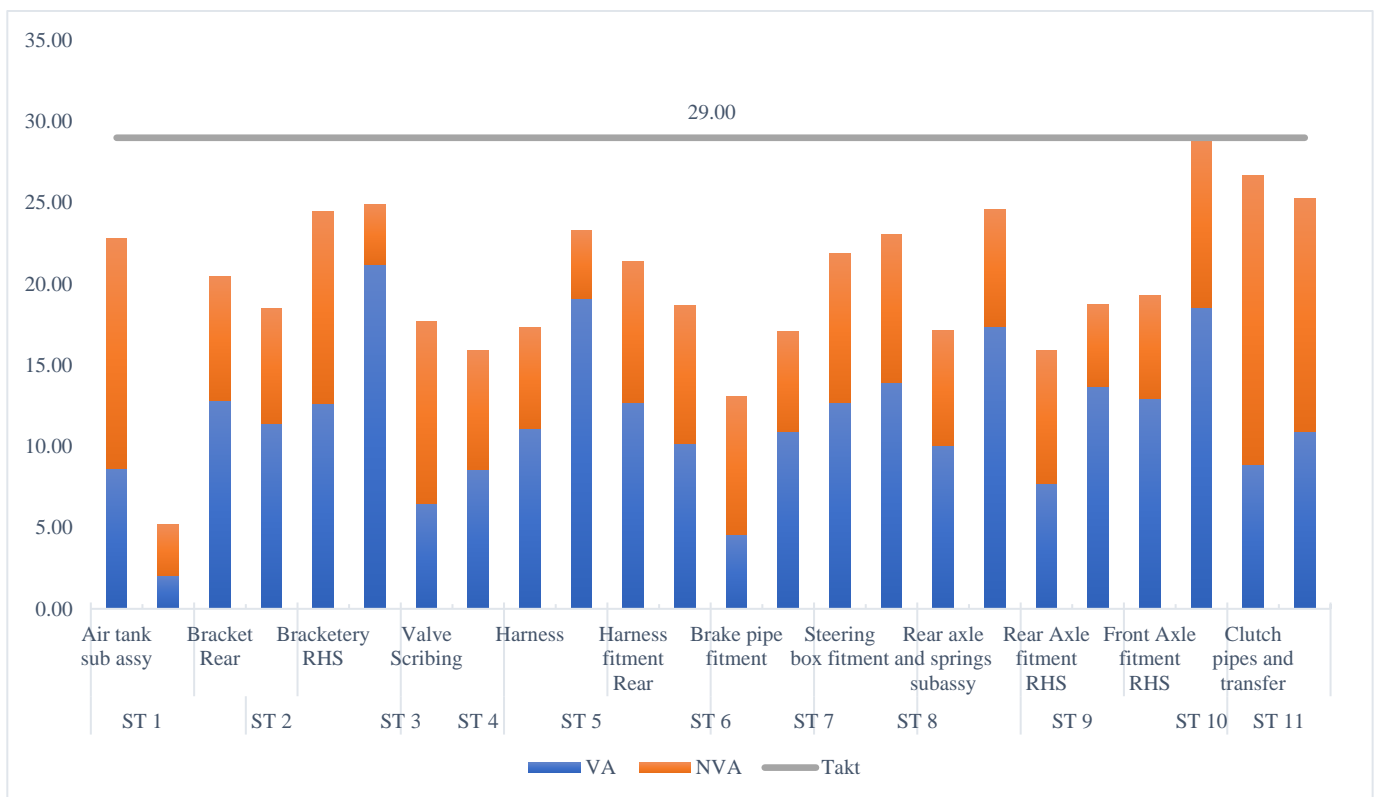
Figure 2. Initial state of the production line balancing of truck manufacturing industry (VA—value added times; NVA—Non-value-added times; Takt time-metric for production time determination).
