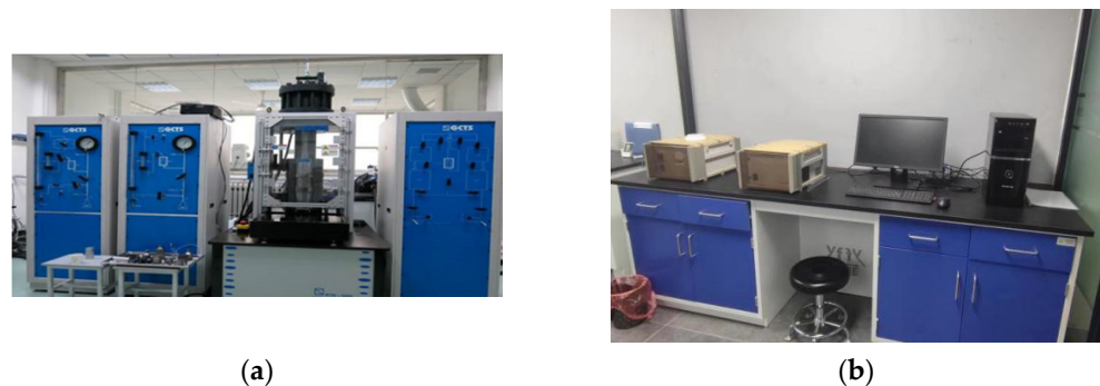
Figure 2. Test equipment. (a) RTR-1000 rock true triaxial mechanics test equipment, (b) RecCore-2513DHNMR test equipment.
