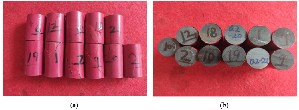
Figure 17. Shale sample after triaxial compression. (a) Shale sample, (b) cross section of shale sample.
