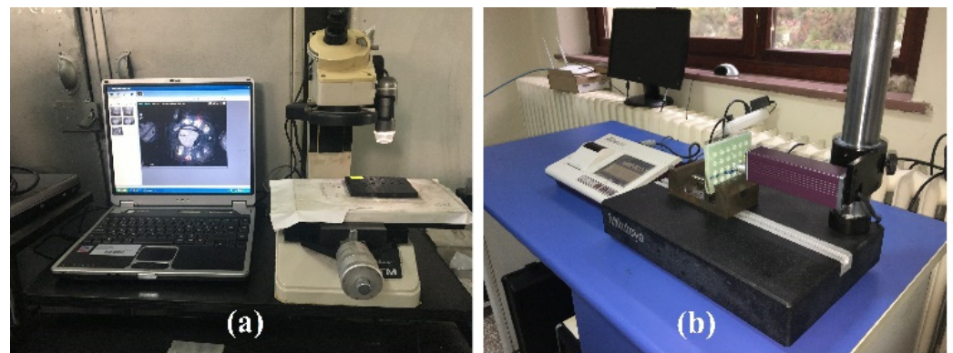
Figure 3. (a) Delamination; (b) surface roughness measurements.
