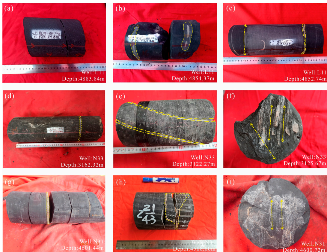
Figure 5. Photographs of fractures and pyrite stripes in shale core samples from three wells. (a) Macro-tectonic fractures, Well: L11, Depth: 4883.84 m; (b) Calcite lenticular bodies, Well: L11, Depth: 4854.37 m; (c) Pyrite inclusions, Well: L11, Depth: 4852.74 m; (d) Horizontal fracture, Well: N33, Depth: 3162.32 m; (e) Highly angular tectonic fractures, Well: N33, Depth: 3122.27 m; (f) Calcite veins adhering to the surface, Well: N33, Depth: 3125.67 m; (g) Pyrite interlayer, Well: N31, Depth: 4601.44 m; (h) Netted cracks, Well: N31, Depth: 4588.80 m; (i) Mirror scratches, Well: N31, Depth: 4600.72 m.
