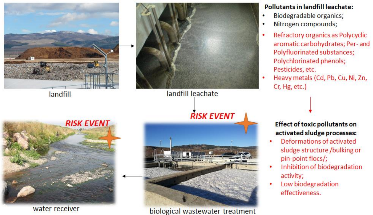
Figure 1. Risk events during biological purification of landfill leachate in wastewater treatment plants. The text, marked in red, indicates risk events that may occur as a result of availability of toxic compounds or refractory organics in the landfill leachate.
