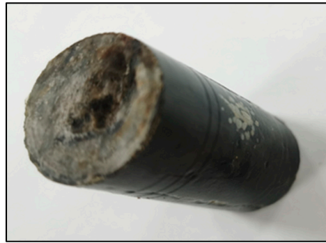
Figure 8. Morphology of the core after dissolution.
