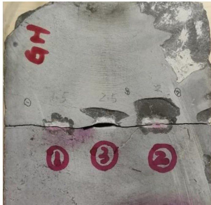
Figure 16. Rock sample split along connected cracks.
