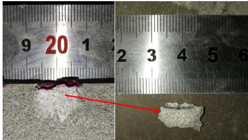
Figure 22. Damaged area generated with wedge tooth in sandstone.
