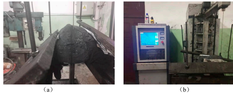
Figure 1. Yarn Cutting Machine (a) Fixed coal sample; (b) Sample take-up.
