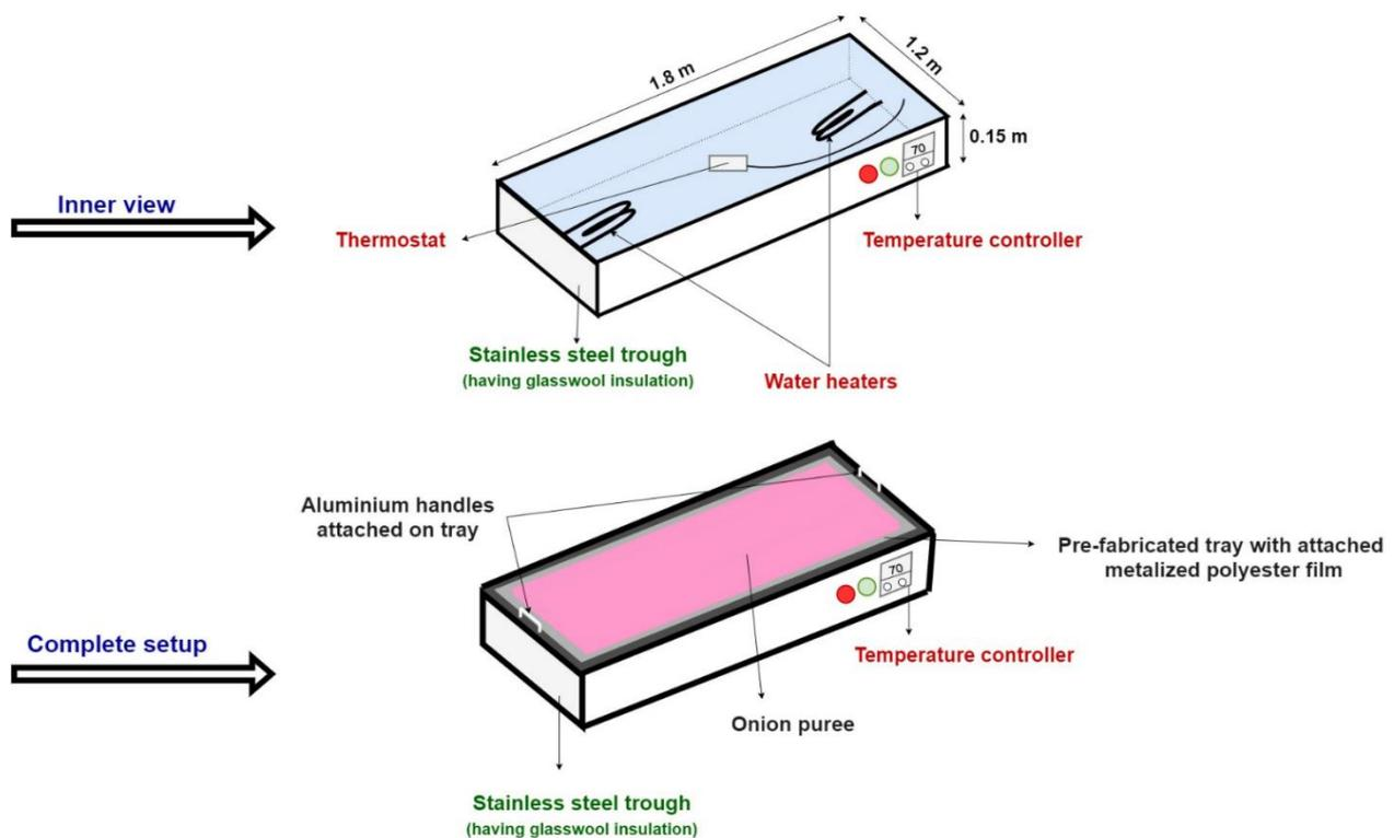
**Figure 1.** Schematic diagram of the refractance window dryer.
