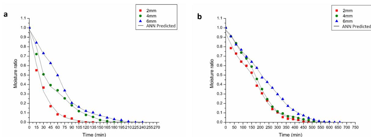
**Figure 6.** Model prediction through ANN and experimental data of moisture ratio of (a) RW dryer and (b) convective dryer.
