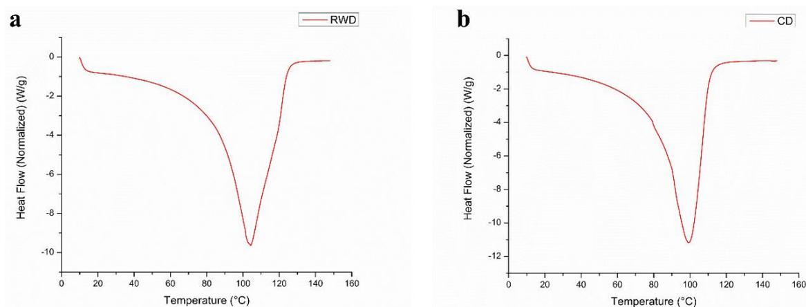
**Figure 8.** Thermal analysis of (a) RW-dried and (b) convective-dried onion powder.
