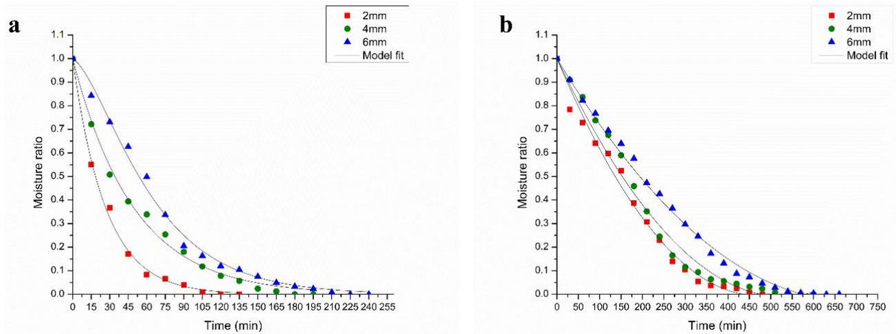
Figure 3. Moisture ratio vs time with best-fit model line: (a) RW dryer and (b) convective dryer.
