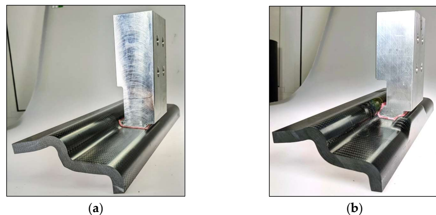
Figure 10. Subcomponent specimens as (a) “basic joint”; (b) “form-fitted joint”.
