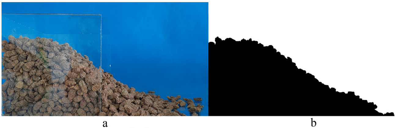
Figure 8. Piling test: (a) photograph of the piling test; (b) image binarization [22].
