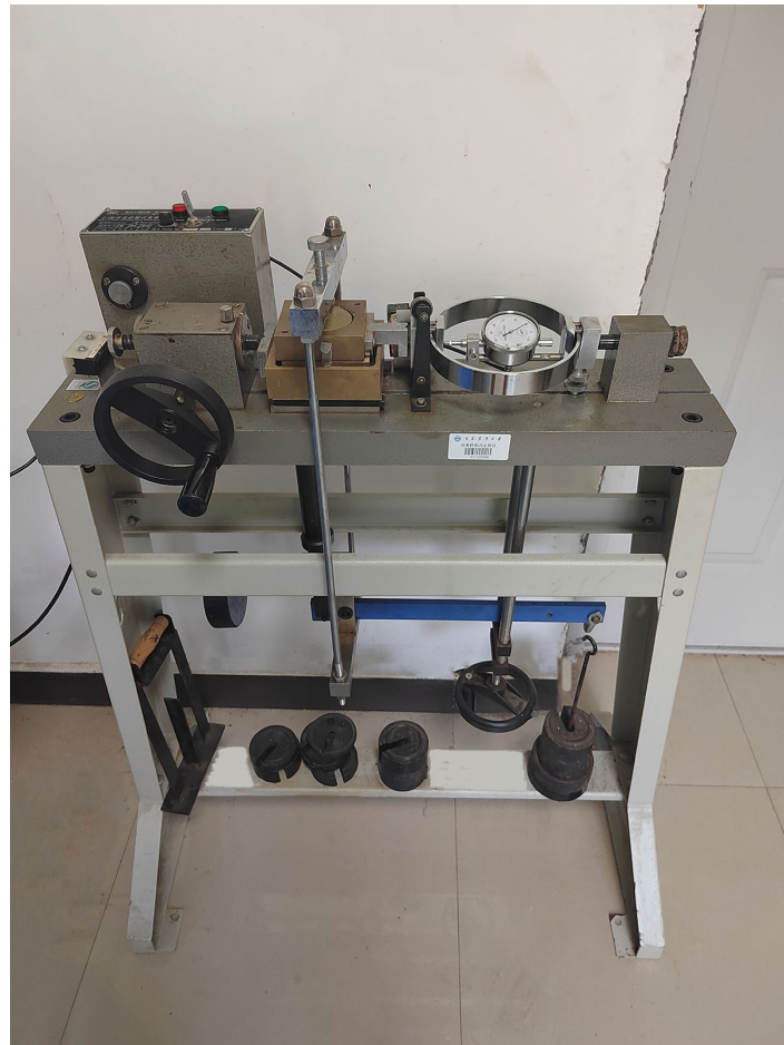
Figure 7. ZJ strain-controlled direct shear apparatus [22].
