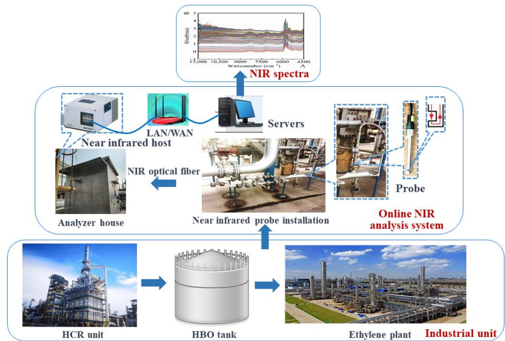
Figure 1. Sampling site and online method for measuring the NIR spectra of the HBO samples.
