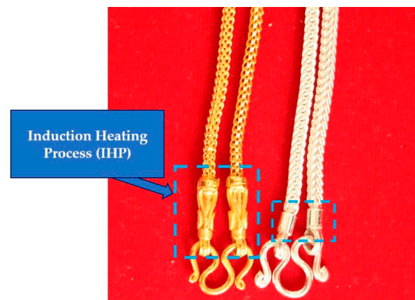
Figure 1. Gold and silver necklaces manufactured from the IHP of a jewelry factory.
