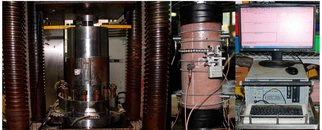
**Figure 3.** XTR01-01 micro-computer-controlled electro-hydraulic servo rock triaxial tester.
