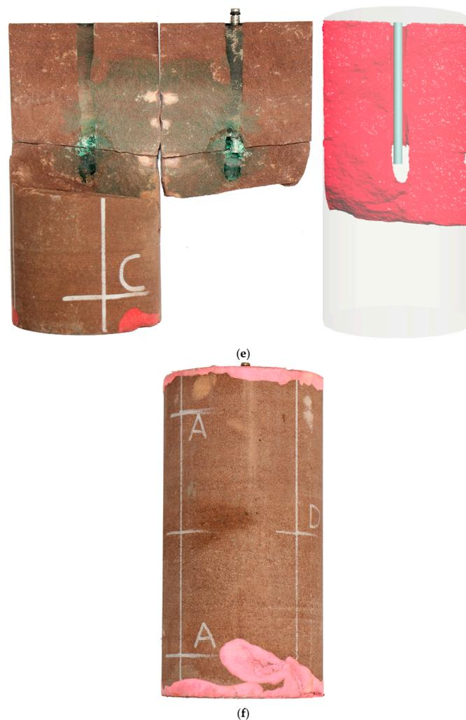
**Figure 13.** Post-fractured view and scanning reconstruction of hydraulic fracture morphology of cyclic hydraulic fracturing samples: (a) S5, (b) S6, (c) S7-1, (d) S10, (e) S13-1, (f) S14-1.
