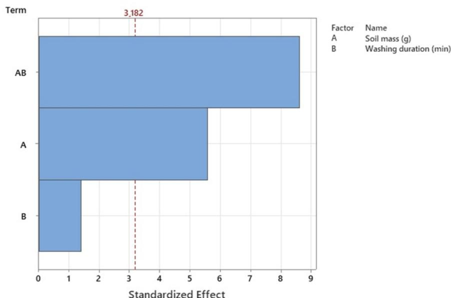
**Figure 7.** Pareto Chart of the standardized effects of Soil mass and Washing duration on the oil removal (%).
