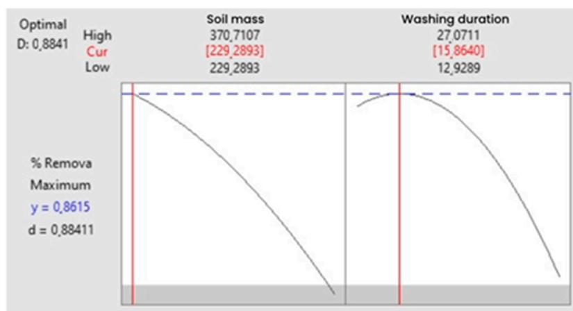
Figure 13. Multiple response prediction for optimization of oil removal (%) by the desirability function related to the Central composite rotational design (CCRD).
