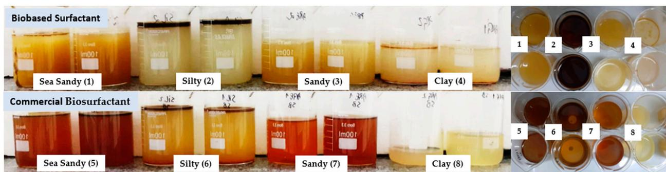
**Figure 17.** Images of surfactants washing solutions after contaminant removal from soils through static treatment. The removal of motor oil from the contaminated soil was carried out through the saturation of 100 g of soil with 10 g of motor oil.
