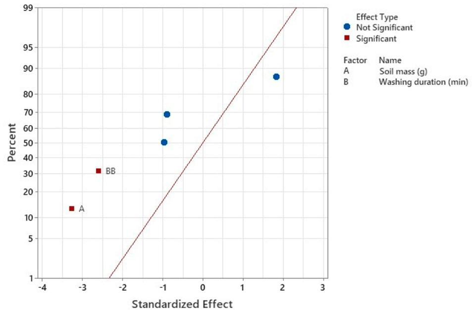
Figure 10. Normal plot of the standardized effects on oil removal (%);  $\alpha$  (significance level) = 0.05.
