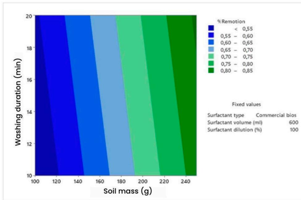
Figure 5. Contour plot of oil removal (%) vs. Soil mass (g) and Washing duration (min).
