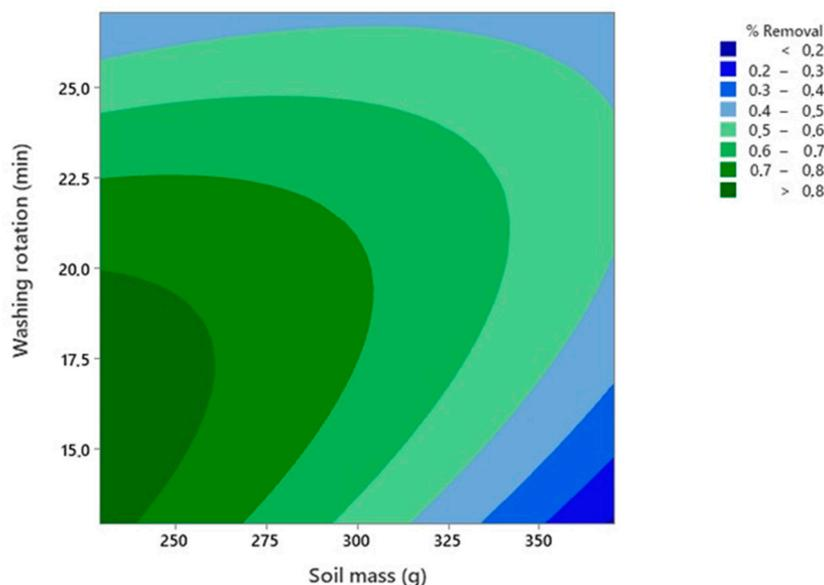
Figure 12. Contour plot of oil removal (%) vs. Washing duration (min) and Soil mass (g).
