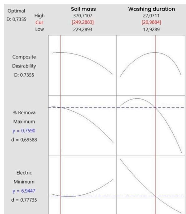
**Figure 15.** Multiple response prediction for simultaneous optimization of oil removal (%) and energy consumption related to the Central composite rotational design (CCRD).
