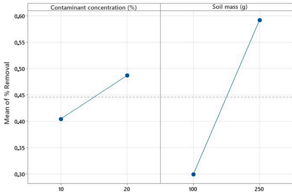
Figure 4. Main effects plot for oil removal (%) (fitted means).
