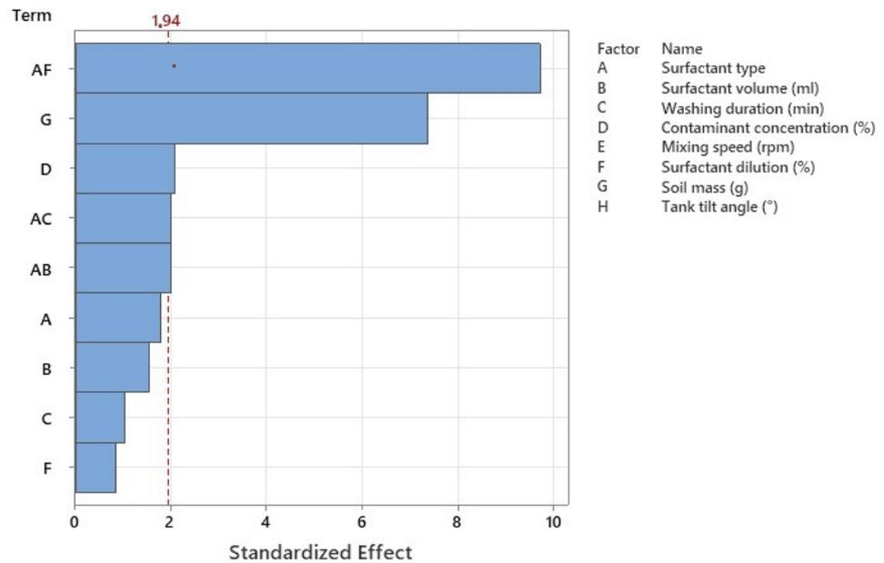
Figure 3. Pareto Chart of the standardized effects of the independent variables on the oil removal (%),  $\alpha = 0.1$ .
