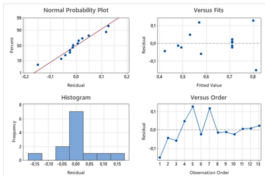
Figure 11. Residual plots for oil removal (%).
