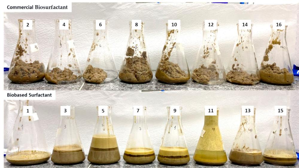
**Figure 2.** Images of solid portion after the experiments of motor oil removal (solid part: sand + non-removed contaminant). Numbers (1–16) correspond to experimental runs performed in  $2^{8-4}$  Fractional Factorial Design.
