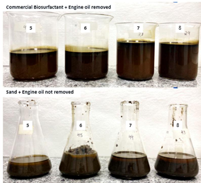
**Figure 14.** Images of washing solutions containing commercial surfactant (**top**) and sand (**bottom**) after axial runs of contaminant removal carried out according to the Central composite rotational design (CCRD) design. Numbers (5–8) correspond to experimental runs.
