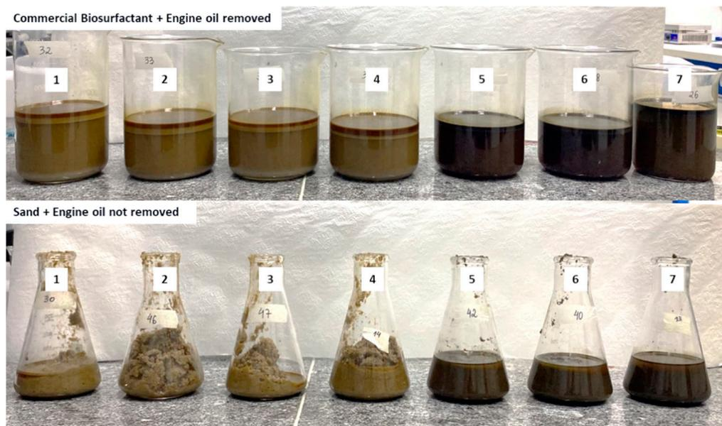
**Figure 9.** Images of washing solutions containing commercial surfactant (**top**) and sand (**bottom**) after contaminant removal runs carried out according to the full factorial design. Numbers (1–7) correspond to experimental runs.
