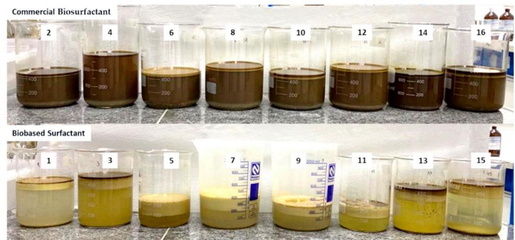
**Figure 1.** Images of surfactants washing solutions after the experiments of motor oil removal (liquid part: sand + removed contaminant). Numbers (1–16) correspond to experimental runs performed in  $2^{8-4}$  Fractional Factorial Design.
