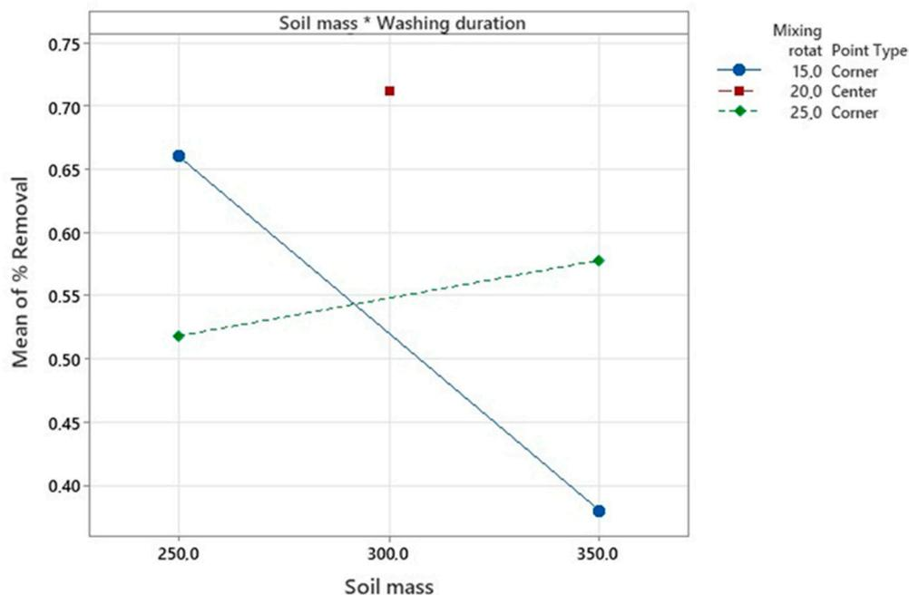
**Figure 8.** Interaction plot for oil removal (%) (fitted means). Soil mass \* Washing duration refers to the interaction effect between these two variables.
