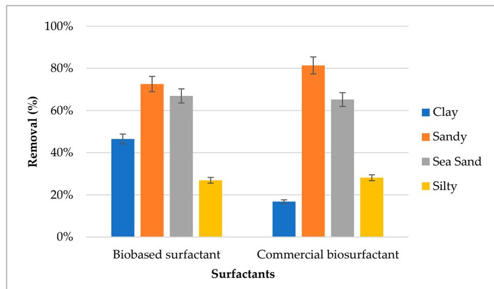
**Figure 16.** Removal of motor oil adsorbed to four types of soils in SRMS using both the biobased surfactant and the commercial biosurfactant.
