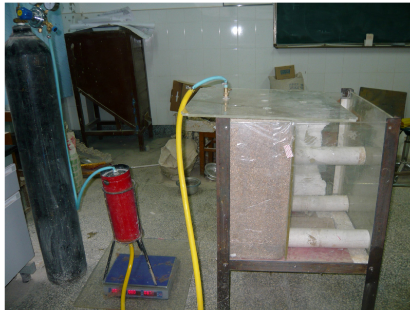
Figure 4. Photograph of the grouting experimental device.
