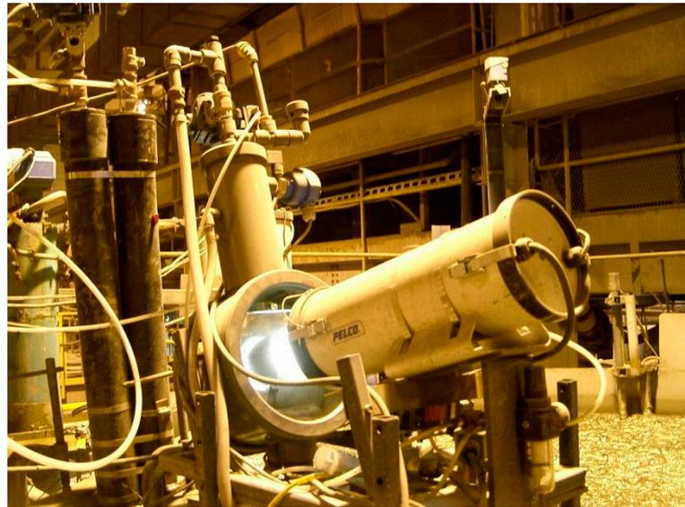
**Figure 2.** Bubble viewer setup on the flotation vessel.
