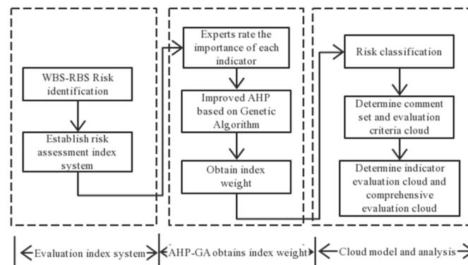
**Figure 1.** Flow chart of risk assessment for immersed tube tunnel construction.
