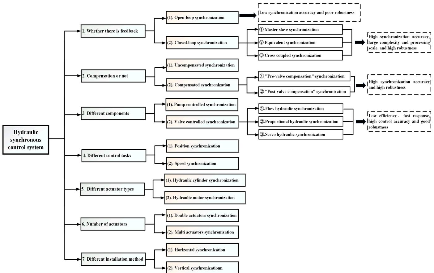
**Figure 1.** Classification diagram of hydraulic synchronous control system.
