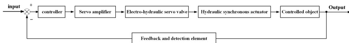
**Figure 8.** Block diagram of electro-hydraulic servo hydraulic synchronization control system.
