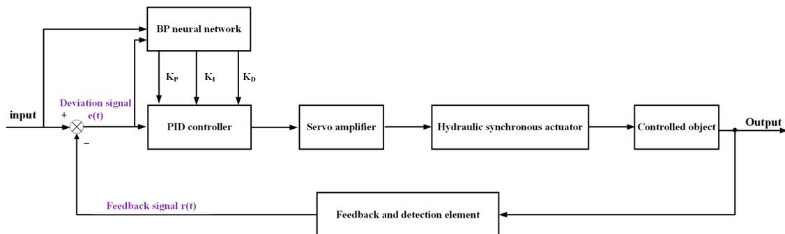
**Figure 12.** PID control principle under BP neural network.
