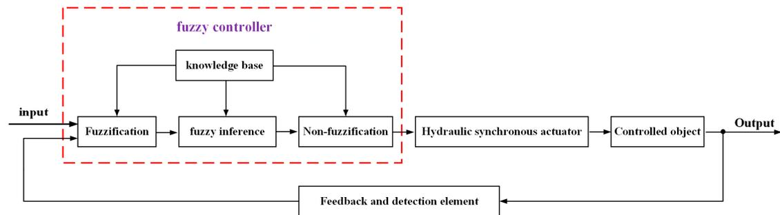
**Figure 9.** Fuzzy control block diagram of hydraulic synchronization control system.
