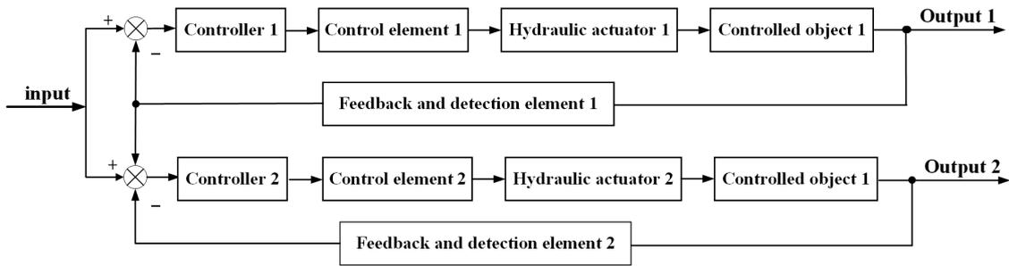
Figure 3. Master–slave control block diagram of hydraulic synchronous control system.
