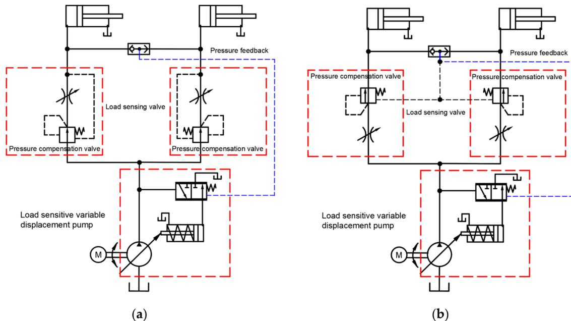
**Figure 6.** Schematic diagram of compensated hydraulic synchronous control system. (a) Schematic diagram of pre-valve compensation hydraulic synchronization control system; (b) Schematic diagram of post-valve compensation hydraulic synchronization control system.
