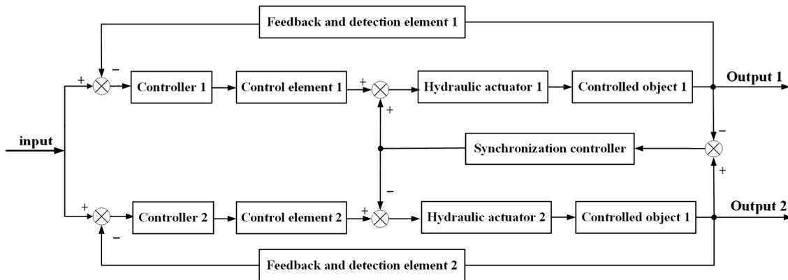
Figure 4. Cross-coupling control block diagram of hydraulic synchronous control system.
