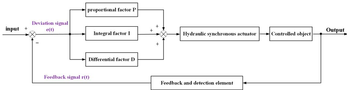
**Figure 10.** PID control block diagram of hydraulic synchronization control system.
