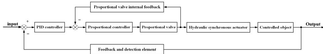
**Figure 7.** Block diagram of electro-hydraulic proportional hydraulic synchronization control system.
