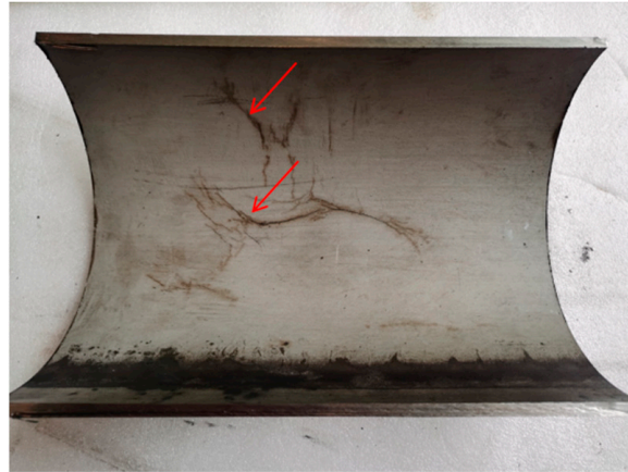
Figure 3. Macroscopic appearance of cracks on the internal surface (The arrows point to the cracks).
