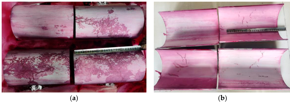
Figure 5. Macroscopic appearance of the pipeline sample after penetration testing: (a) external wall; (b) internal wall.
