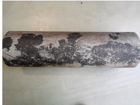
Figure 1. Macroscopic morphology of the pipeline sample.
