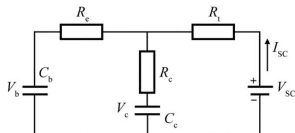
Figure 2. Supercapacitor RC model.
