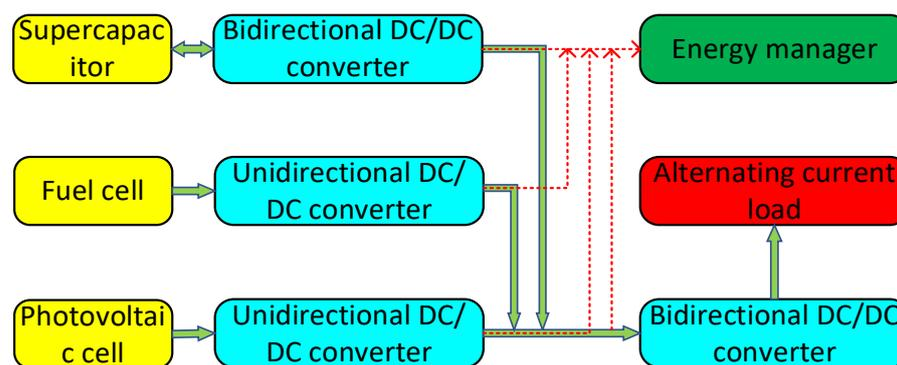
**Figure 1.** Integrated energy and power supply system topology based on fuel cells.
