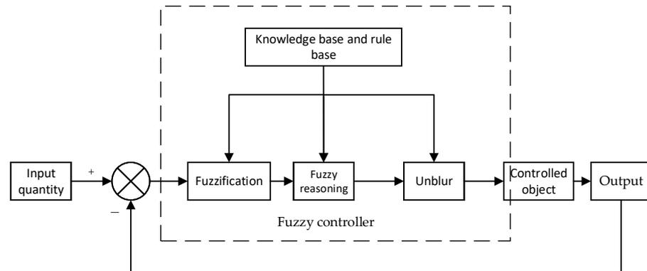
**Figure 3.** Structure diagram of fuzzy logic control system.
