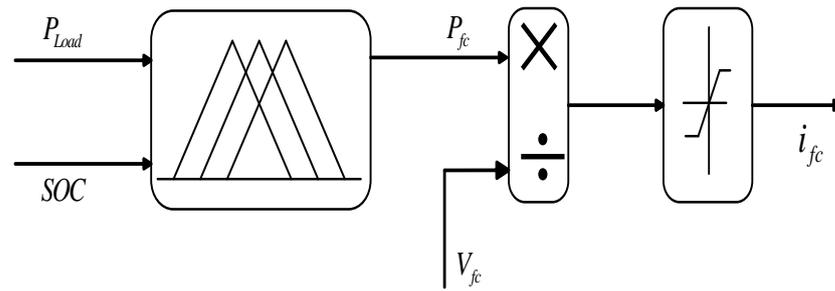
Figure 4. Designing a fuzzy-logic controller.
