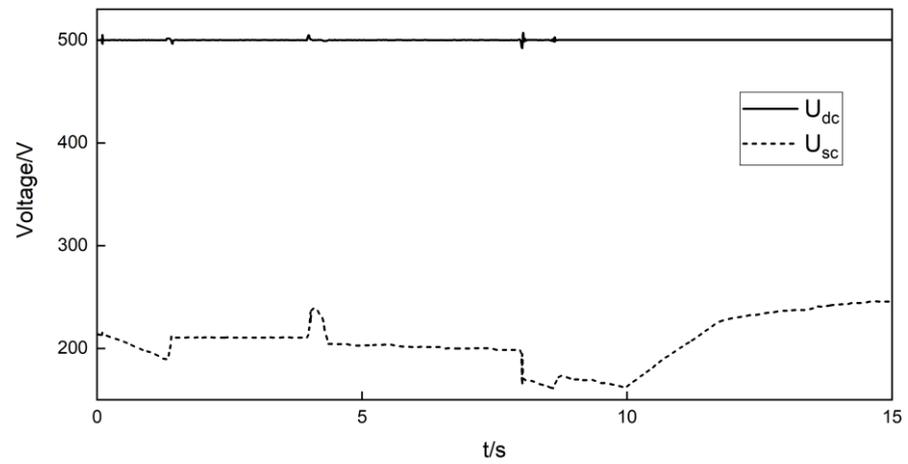
Figure 8. Ultracapacitor voltage and DC bus voltage.
