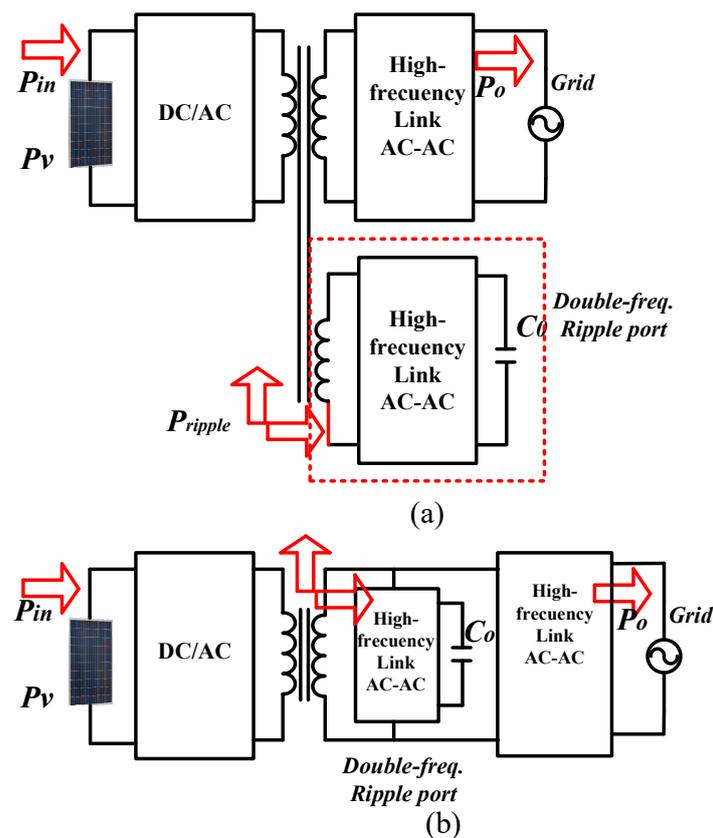
**Figure 12.** Approaches to the ripple port connections: (a) ripple port by using the rail voltage indirectly; (b) ripple port by using the rail voltage directly [78].
