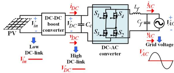
Figure 5. Single-phase grid-connected scheme [64].
