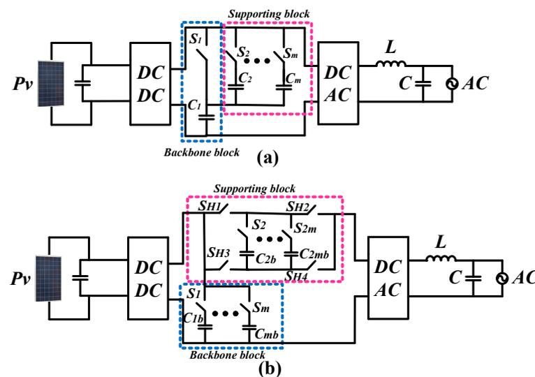
Figure 3. SSC architectures: (a) unipolar; (b) bipolar [57,58].
