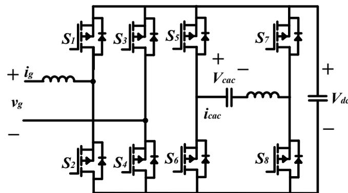
Figure 10. Capacitive energy storage with a full-bridge inverter.
