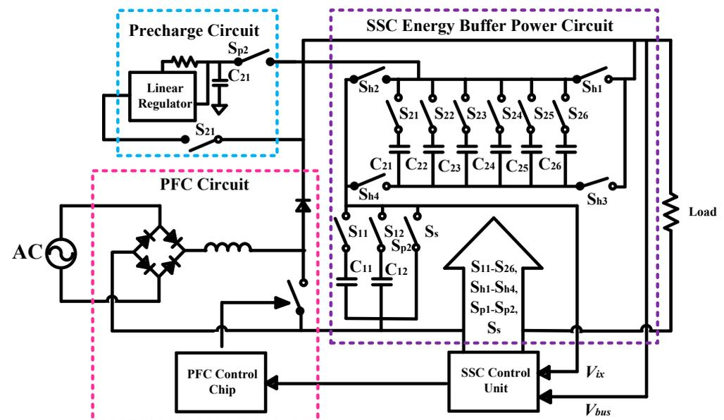
**Figure 7.** SSC energy buffer system: pre-charge circuit, SSC energy buffer, SSC control unit, and PFC circuit [66].
