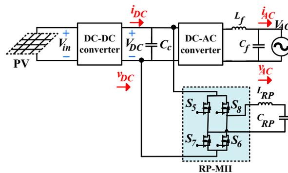
Figure 6. Single-phase grid-connected structure by applying an RP-MII [64].
