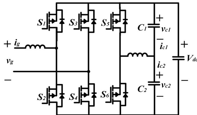
Figure 9. PWM rectifier system with two capacitors as energy storage elements.
