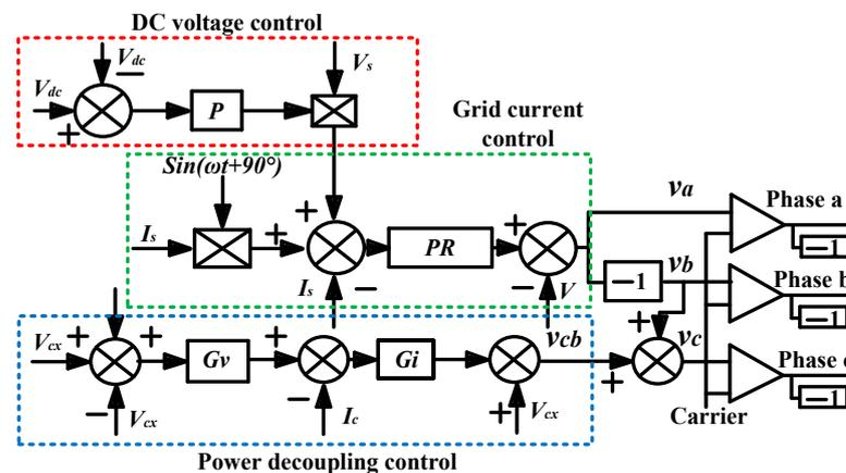
Figure 11. Control to proposed active power decoupling.
