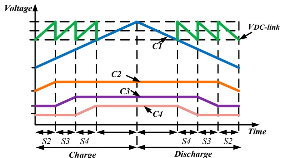
Figure 4. States of commutation of unipolar SSC [60].
