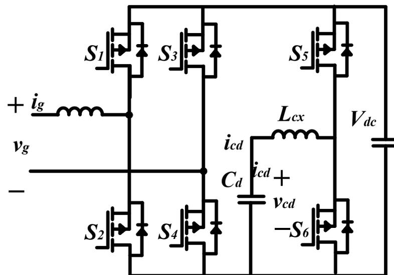
**Figure 8.** Capacitor energy storage in bipolar mode [71].
