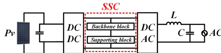
Figure 2. Basic scheme by applying an SSC architecture.
