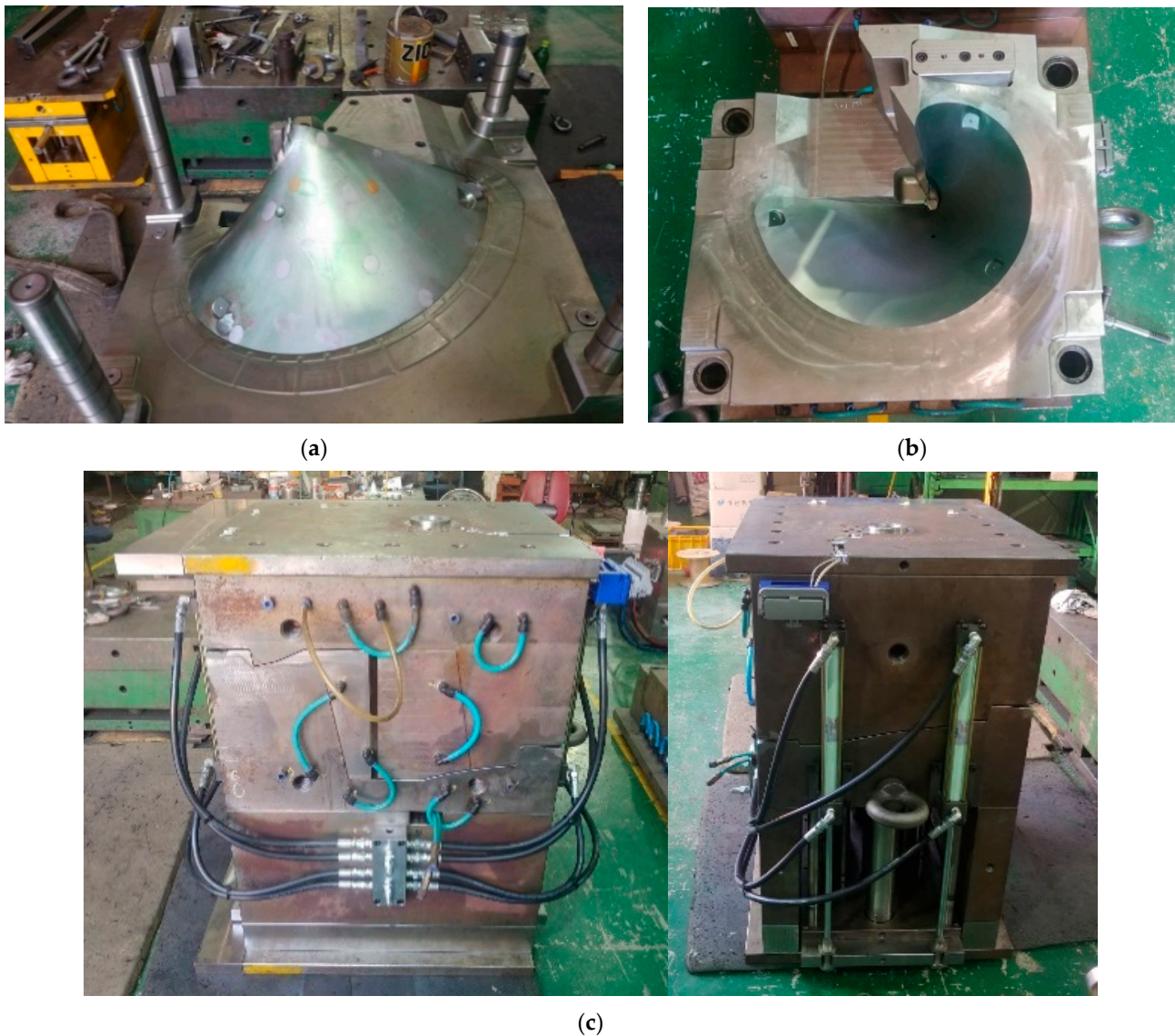
Figure 17. Photographs of the manufactured mold. (a) Mold movable side; (b) Mold fixed side; (c) Mold assembly with cooling channels.
