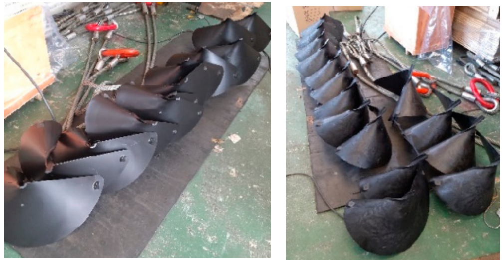
Figure 18. Blades manufactured by test injection molding.
