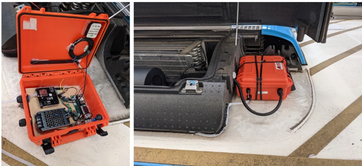
Figure 5. Installing a COCAL box on buses.
