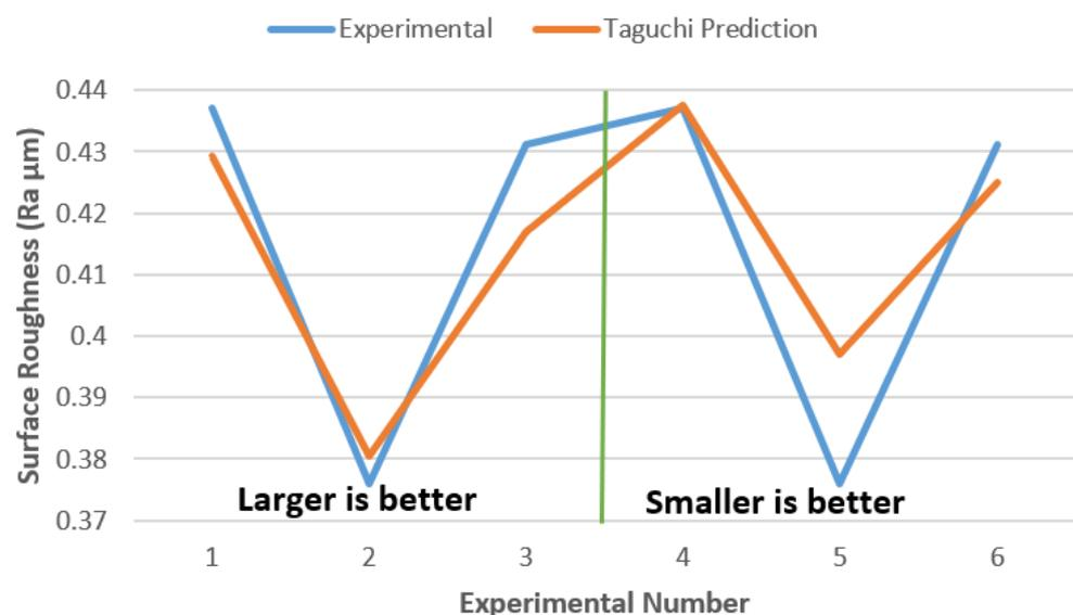
**Figure 4.** Comparison of experimental results with predicted values.
