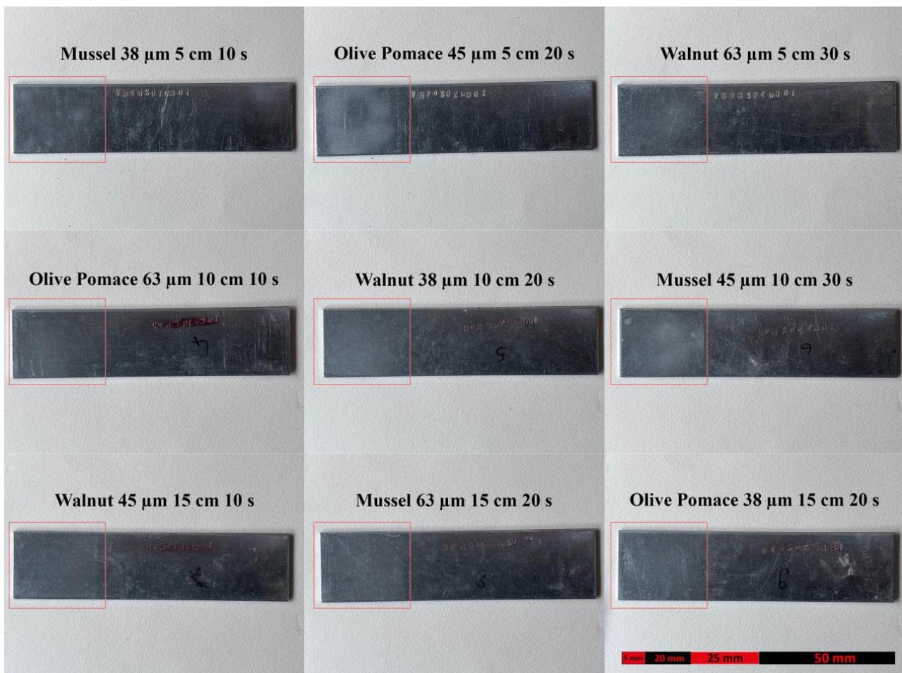
**Figure 5.** Surface images of samples after abrasive blasting.
