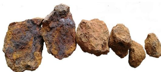
**Figure 1.** Raw gossan ore sample.
